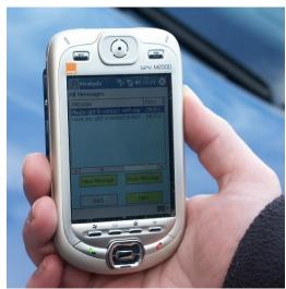
VTRAKPDA is a software application that sits on a PDA device that has GPRS connectivity. These devices, as well as giving data communications allow for drivers to make telephone calls and take photos of the vehicles they attend, as these devices are "Of the shelf" they can be bought from your mobile communications provider where they can be bulk purchased for very little money.
