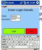
The driver logs into the PDA with their own unique username and password. This logs them into the VTRAK system back in the control room and shows them as an "Active" driver within VTRAK.
