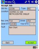
The driver can alter the ETA time to scene and then presses the "Accept" button to notify the control room that he is on route to the job.
