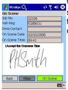
When the driver arrives with the customer. The customer is asked to sign the screen to acknowledge that the driver arrived on scene at the time shown. The driver then presses the "Onscene" button to notify the control room of his status.
